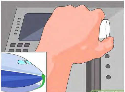
5 Reduce the throttle to idle. Raise the nose slowly by pulling back on the yoke, until the two main wheels touch down. Continue holding the nose wheel off the ground; it will settle to the ground by itself.
